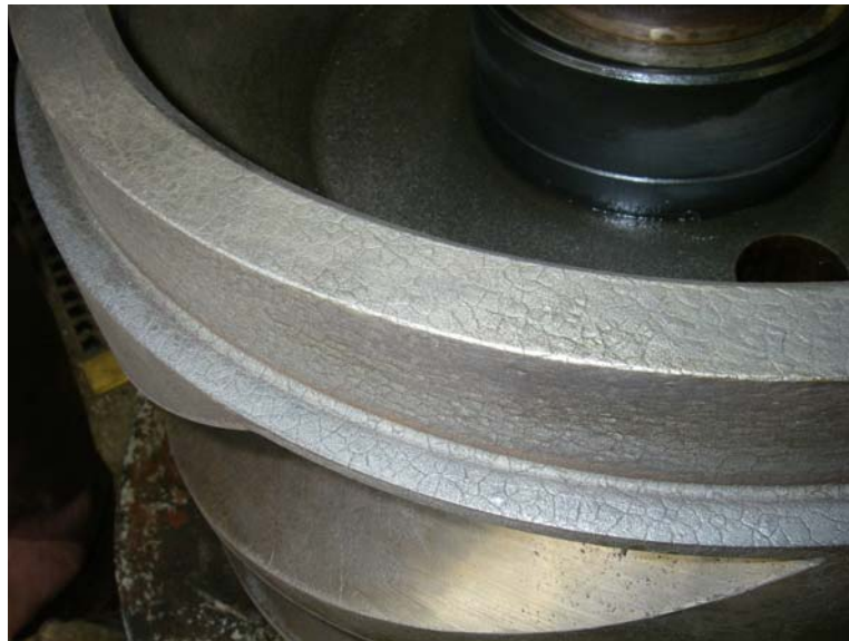
Figure 5. Etching of the main single screw rotor after being exposed to severe refrigerant - sulfuric acid - water conditions for a 100 hours running period.
