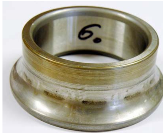
Figure 3B. Super-tough stainless steel ring (AMS 5898) from a thrust bearing in hydrogen rich service. About 8000 hours of service (some light stains).
