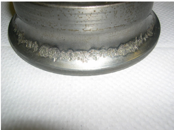
Figure 3A. Steel inner ring (conventional AISI 52100) from a thrust bearing used on the main rotor with the raceway spalled (hydrogen attack) and frosted raceways (poor lubrication). Less than 1000 hours in service.
